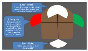
Basic navigation lights required by most vessels including the arc of visibility of each of the lights. Exact placement aboard the vessel depends upon size and design but must be in accordance with Annex I of the Rules (33 CFR 84).
